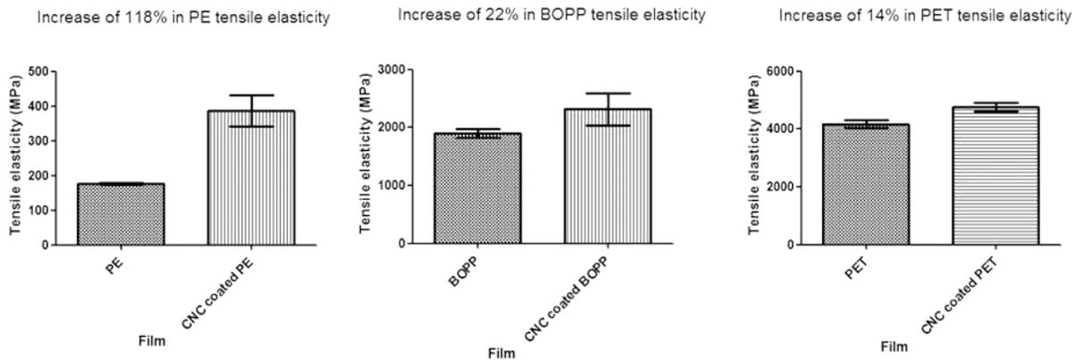
**Fig. 1:** Tensile elasticity comparison of coated and uncoated plastic films
